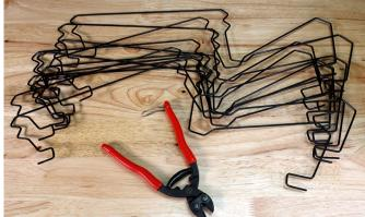
Manually feed a little extra wire before cutting. Leave about 1/2" extra wire at the end of each cross-section. This will be used to insert into the top and bottom plates.
