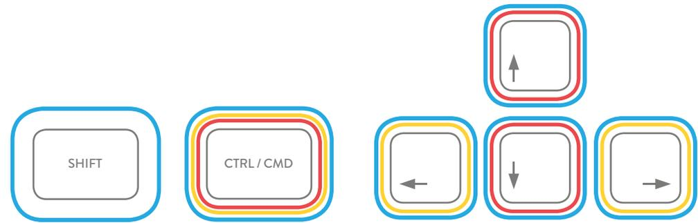
Hold control and press arrow keys to manually move the bend pin or feed the wire. This is helpful loading new wire.
