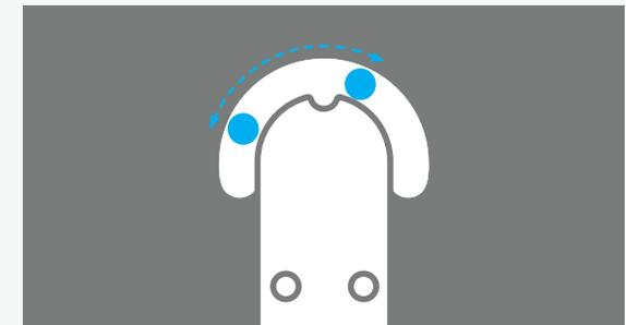
Before bending, the D.I.Wire needs to go through the homing sequence to ensure the bend pin is in the proper position.
