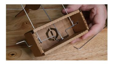
Next, feed the 3 support rods into the box and secure them to the crankshaft with needle-nose pliers. Just a simple pinch of the support wires should hold them in place.
